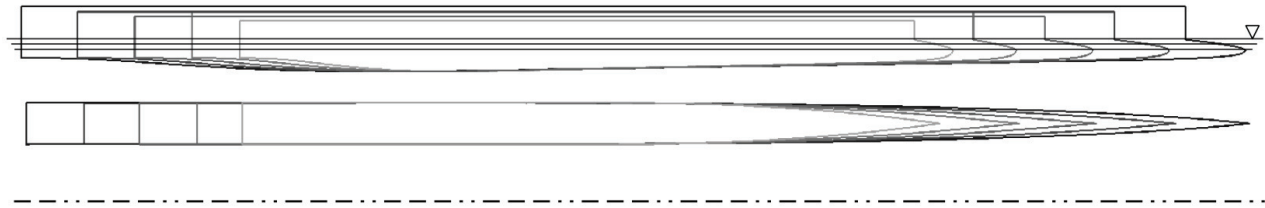
Figure 1: Profile view (top) with corresponding water lines for light, medium and heavy displacement and plan view (bottom) with symmetry line of hulls under consideration.
