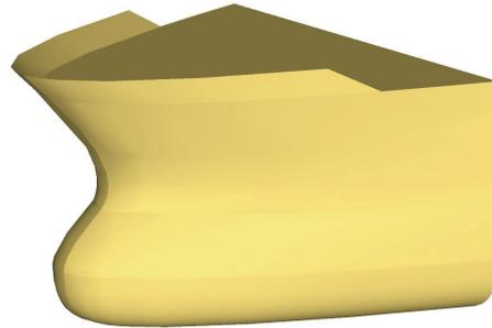
Figure 5: Striking ship bow model: Bulk carrier
