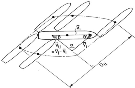
Figure 7: Definition of geometrical collision diameter [32]
