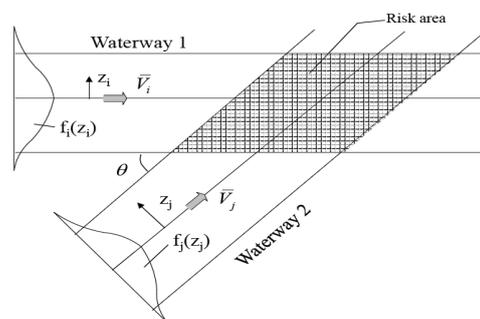
Figure 6: Pedersen's model for intersecting waterways, with a risk area for ship-ship collisions [32]
