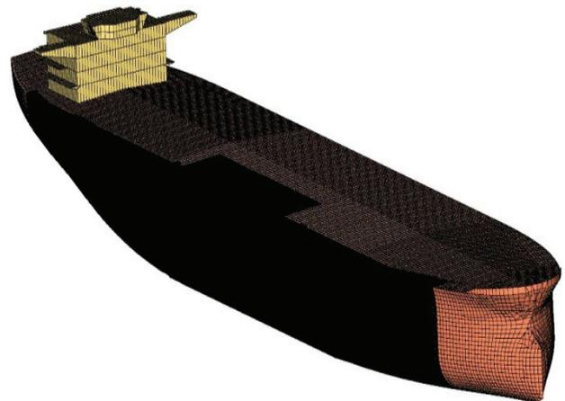
Figure 4: Struck ship finite element model
