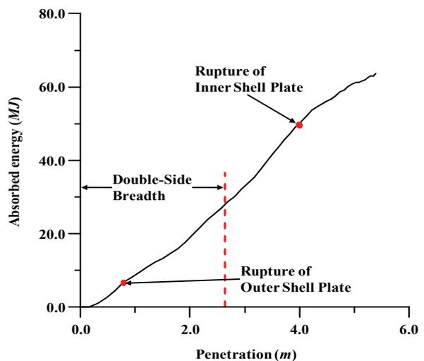
Figure 10: Collision energy absorption versus penetration
