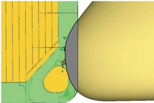
Figure 11: Definition of the structural damaged volume of the struck ship
