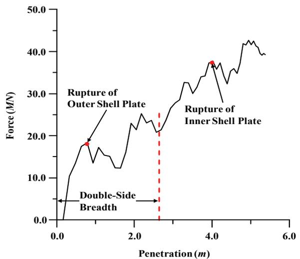
Figure 9: Collision resultant force versus penetration
