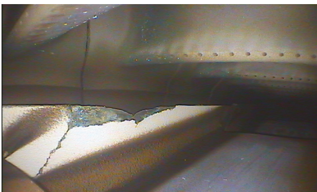
Figure 4: View of damaged thermal protection layer of a rotor blade
