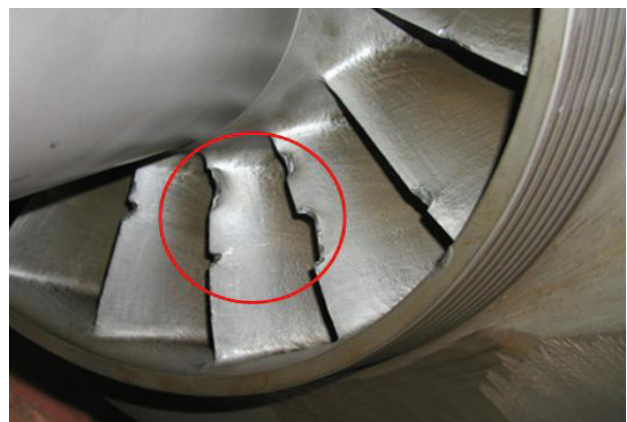
Figure 5: Detailed view of the damaged blades on the first stage of the compressor after disassembly
