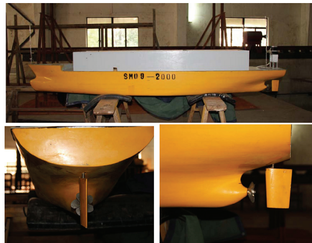
Figure 1- Ship model, propeller and rudder
