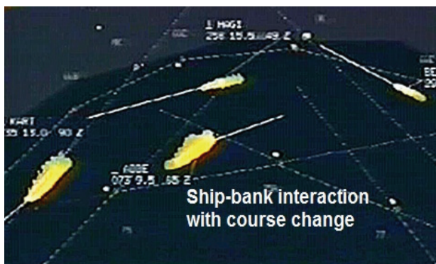
Figure 21 – Ship-bank interaction for an inbound sailing ship on the Western Scheldt
