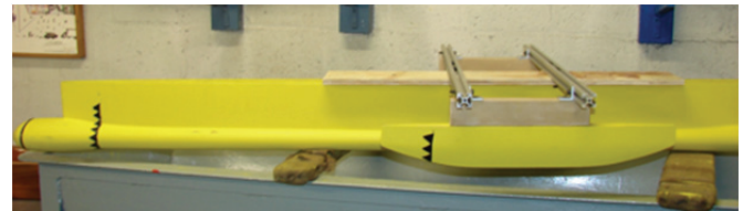
Figure 3 Towing tank Tri-SWATH model used to collect experimental model resistance data [7]
