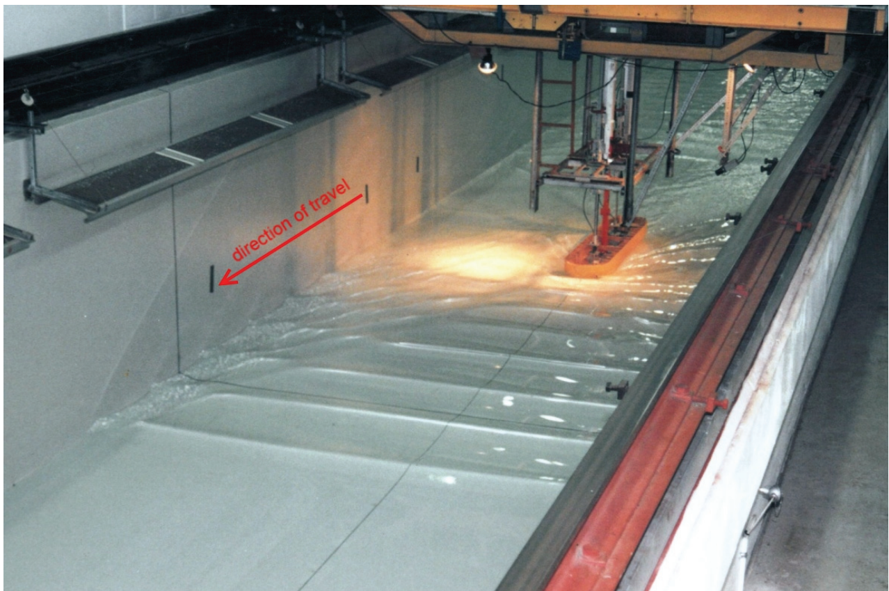
Figure 9 – Solitons generated from a mono hull in the AMC Towing Tank
