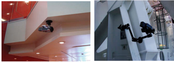
Figure 1. Digital video cameras and mounting options (left: magnetic and right: friction clamp)
