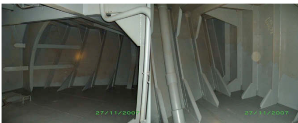
Figure 3: Void Space, between Bosun's store and Forepeak Ballast Tank for Panamax size bulk carrier. (Photos taken by Mr. P. Georgakis).
