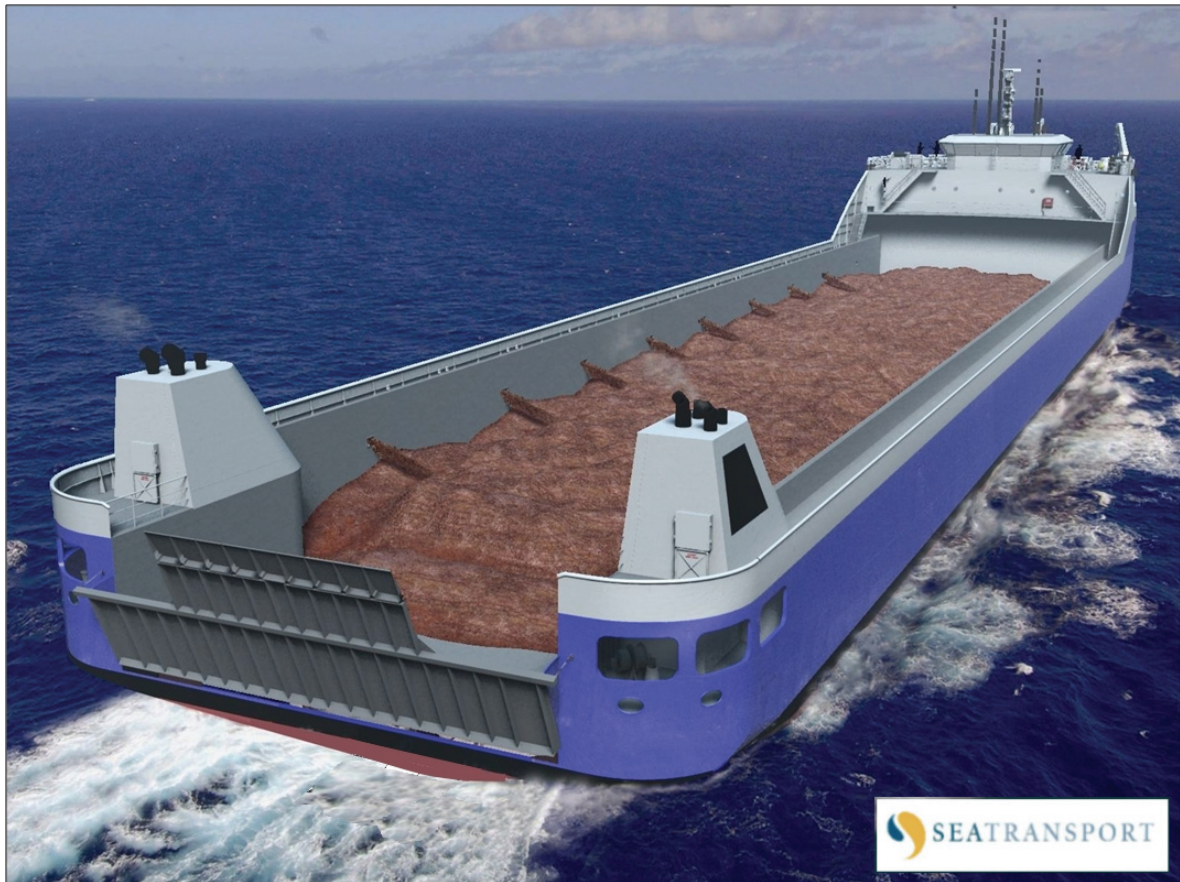
Figure 2 – Stern Landing Vessel – bulk ore cargo
