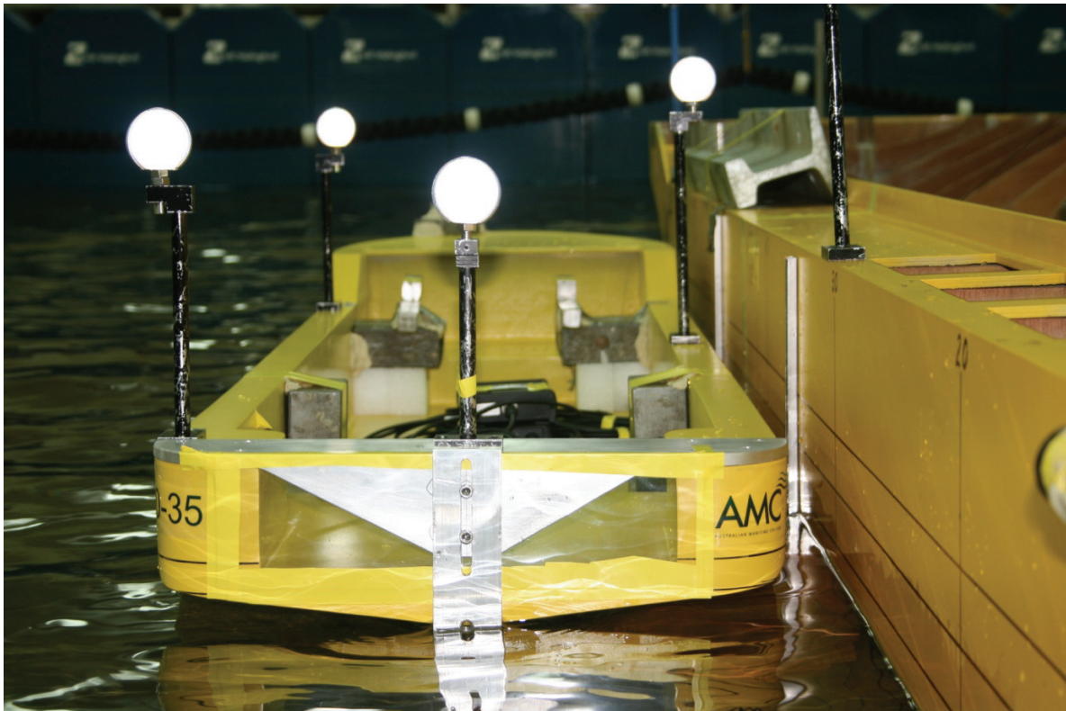
Figure 4 – close up view of the model of the feeder vessel alongside the FHT model
