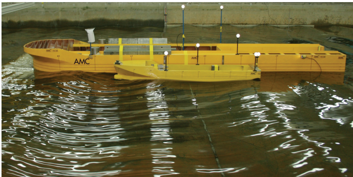
Figure 3 – model tests with the feeder vessel alongside the FHT
