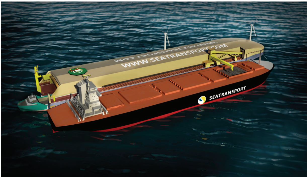
Figure 1 – Floating Harbour Transhipper (mining). An SLV is in the well dock and a Capesize vessel is moored alongside (foreground)
