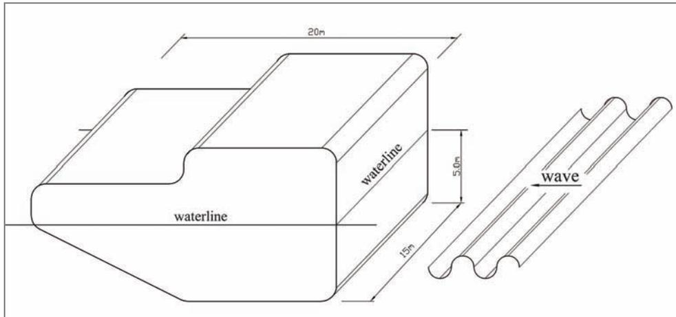
Figure 1: Perspective view of the UGEN wave energy converter
