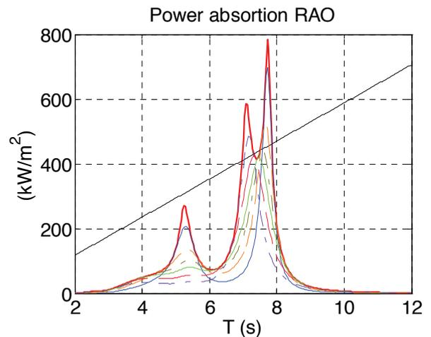
Figure 6: Transfer function of the absorbed wave power for various settings of the PTO (Bpto).
