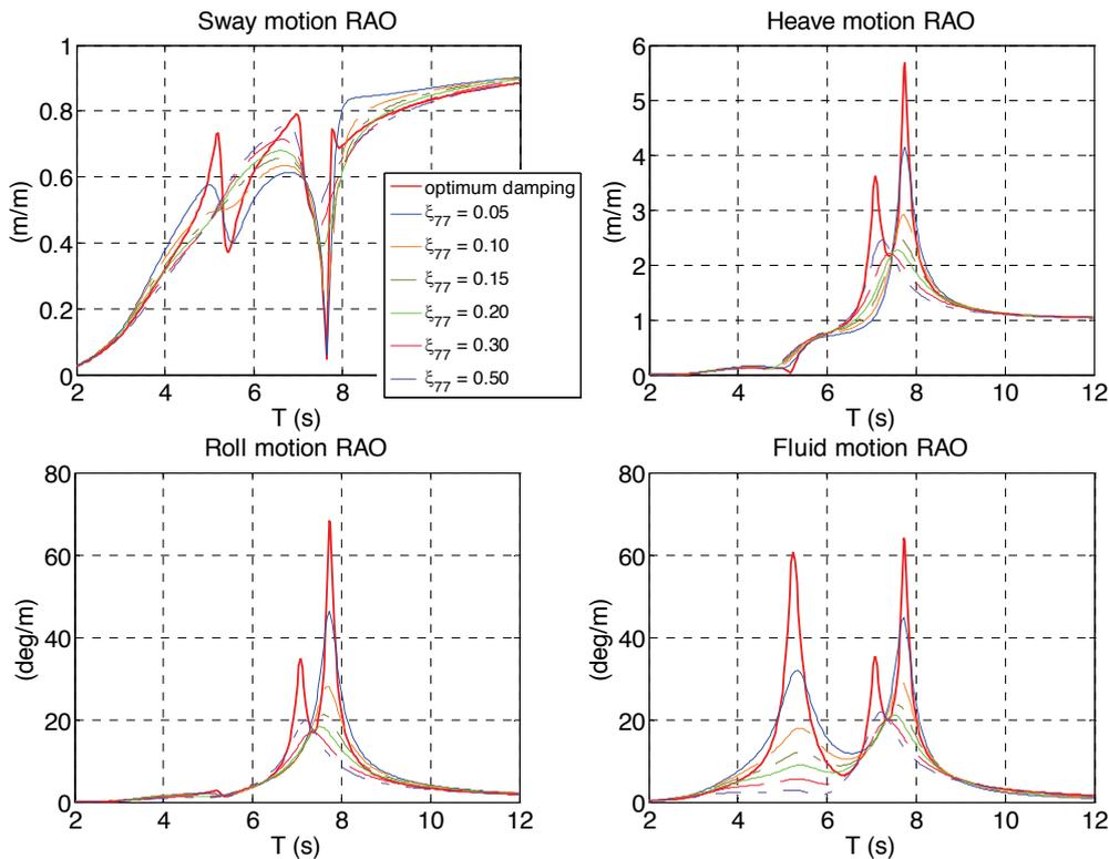
Figure 5: Transfer function amplitudes as function of the PTO setting (Bpto).
