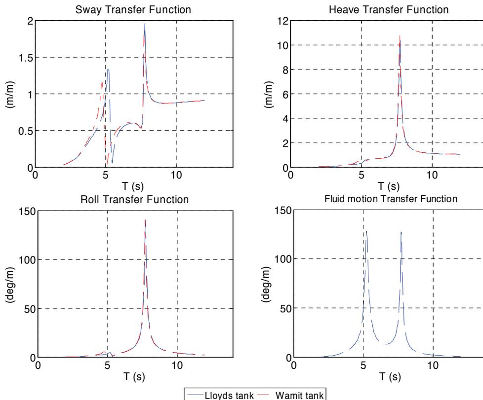
Figure 4: Transfer function amplitudes of the rigid body motions and fluid in the tank motions.
