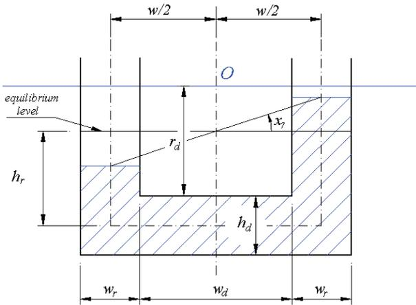
Figure 3: Passive U tank of Lloyd's (1989) method
