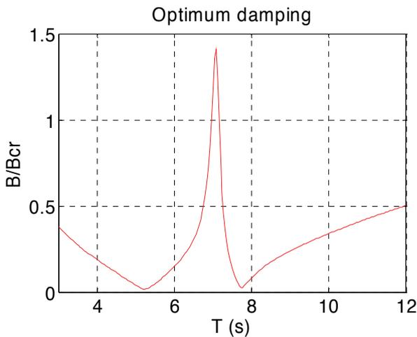
Figure 7: Optimum damping of the PTO
