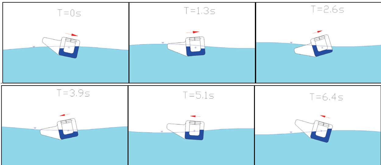
Figure 9: Time sequence of the rigid body motions and fluid motions in harmonic waves with the rolling natural period ( $T = 7.7s$ ).
