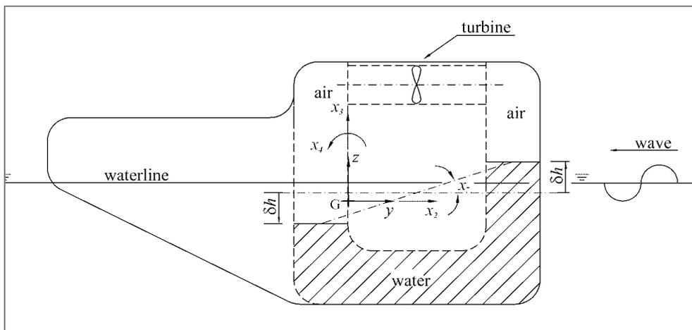
Figure 2: Side view of the UGEN wave energy converter, coordinate system and convention for the motions
