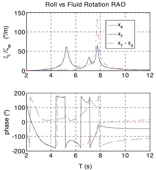
Figure 8: Amplitudes and phases angles of the roll and fluid motions ( $B_{pto}/B_c = 0.05$ )
