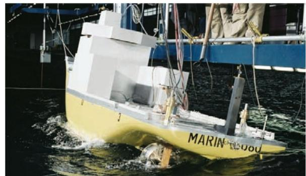
Photograph 8: Propeller ventilation
