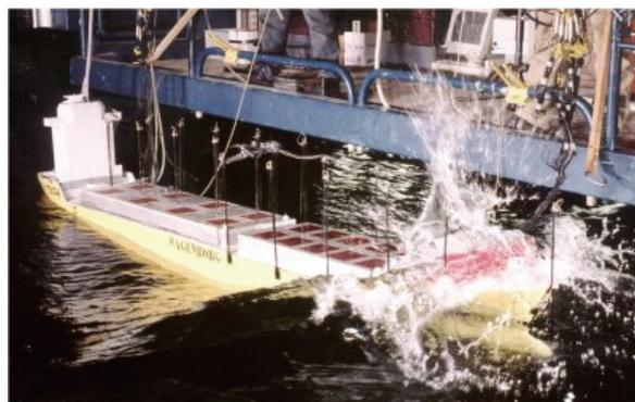
Photograph 2: Breakwater impact in head seas
