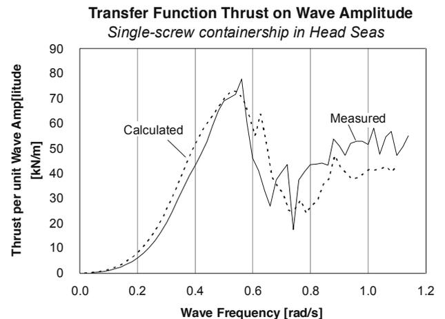
Figure 3: Transfer function of propeller thrust variations
