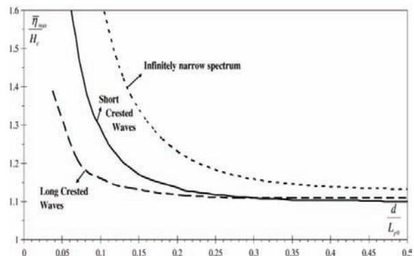
Figure 1: The ratio  $\eta_{max}/H_c$  of the nonlinear and the linear height of the largest wave crest as a function of water depth  $d$ . With  $H_c=8 \cdot \text{R.M.S}$  of wave [3]
