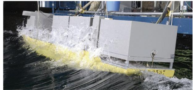
Photograph 5: Impact from a breaking wave from abeam
