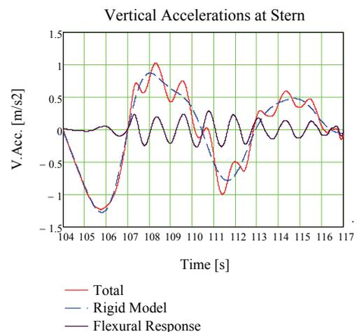
Figure 4: Cruise ship whipping and rigid body accelerations in low waves
