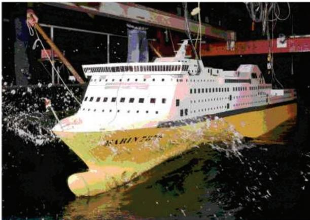
Photograph 1: Seakeeping model of a ferry
