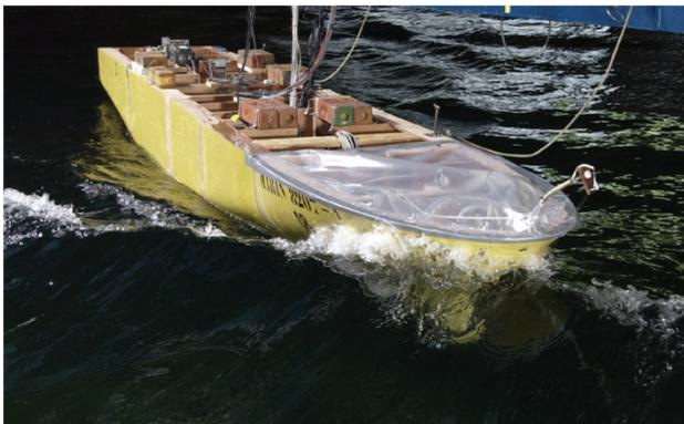
Photograph 4: Bow flare impact from a steep wave from the bow quarter
