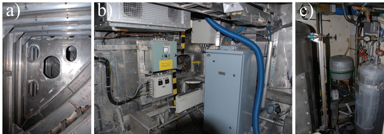
Figure 4: Flooded compartments: a) side tank with anti-sloshing bulkhead, b) equipment room and c) pump room
