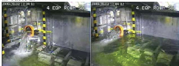
Figure 8: Different flow conditions of the valve between the side tank and the equipment room
