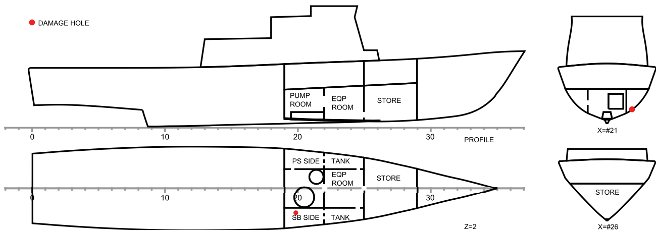
Figure 3: General arrangement of the flooded compartments.
