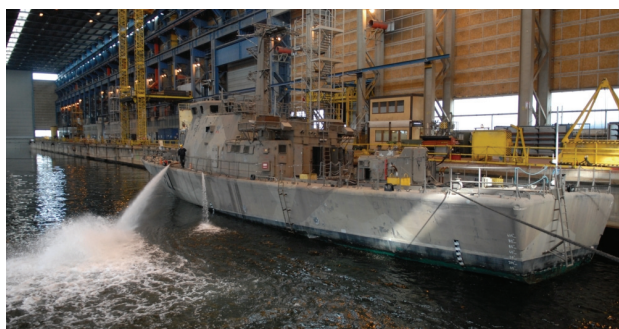
Figure 6: Pumping after a flooding test
