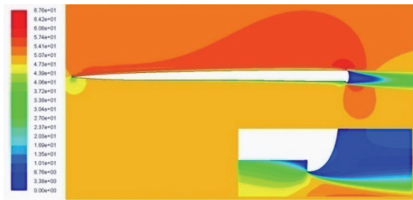
Figure 18: Velocity contours around the blade section of 0.5 R and stagnation zone in front of its spoiler
