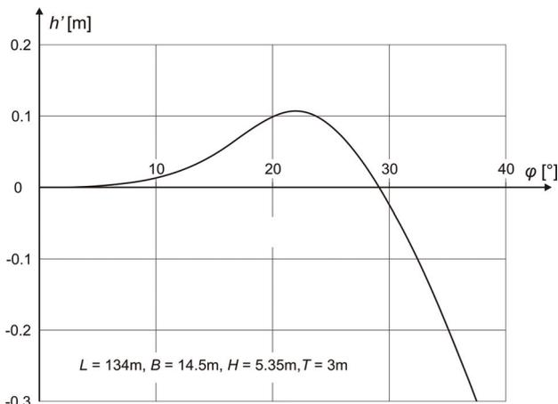
Figure 2: Residual stability lever of the sample vessel
