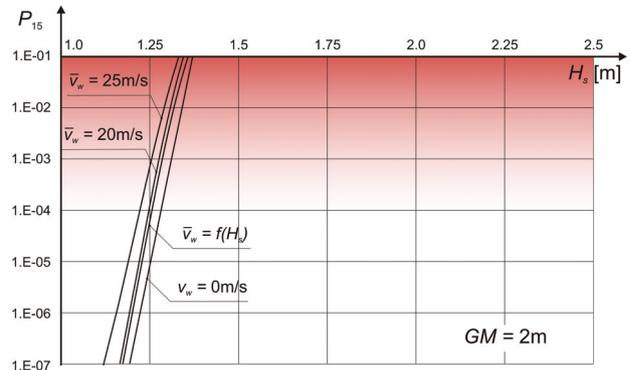
Figure 7: The influence of the beam wind speed on the probability of heeling to 15° for  $GM = 2m$
