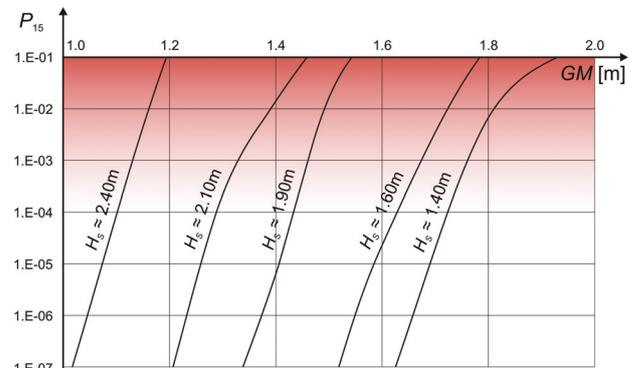
Figure 3: Probability of heeling to  $15^\circ$  vs. metacentric height
