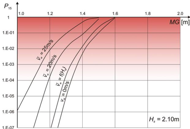
Figure 4: The influence of the beam wind speed on the probability of heeling to 15°
