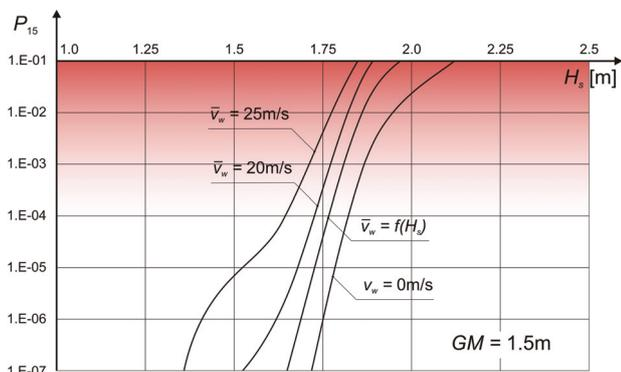
Figure 6: The influence of the beam wind speed on the probability of heeling to 15° for  $GM = 1.5m$
