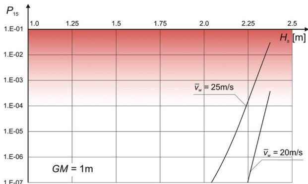
Figure 5: The influence of the beam wind speed on the probability of heeling to 15° for  $GM = 1m$
