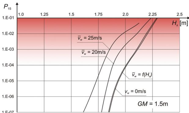
Figure 8: The influence of the beam wind speed on the probability of heeling to 15° for  $GM = 1.5m$ , vessel equipped with bilge keels
