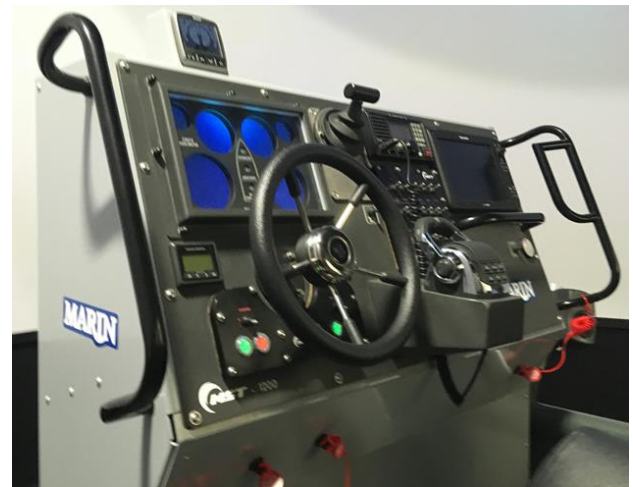
Figure 3: Console with steering wheel, throttle, engine trim and navigation screens situated on the motion base
