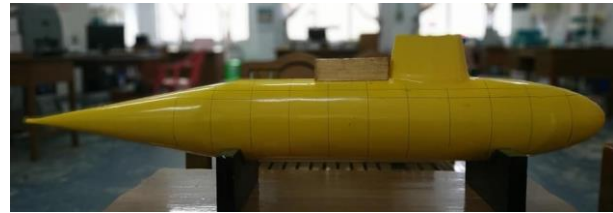
Figure 2: Fabricated wooden model without appendages.
