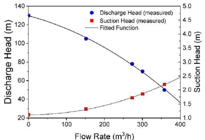
Figure 2. Performance curve of the actual bilge pump
