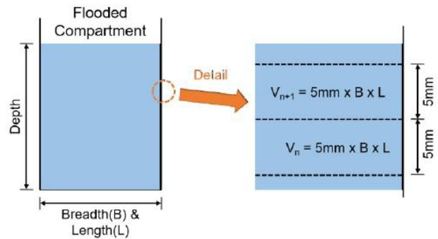
Figure 5. Concept of calculation
