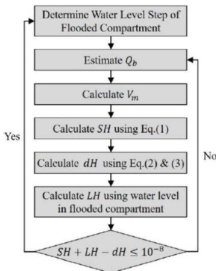
Figure 4. Calculation Procedure
