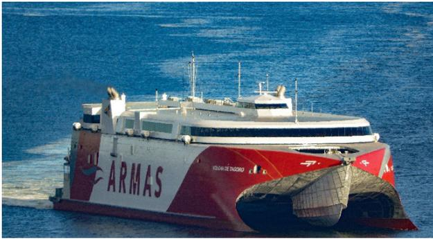
Figure 1. Volcan de Tagoro, Hull 091 111m wave-piercing catamaran built by Incat Tasmania in 2019.
