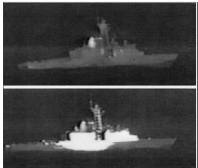
Figure 8: Solar Glint from Typical Navy Grey Paint. Source: Thompson, et al. 2000a
