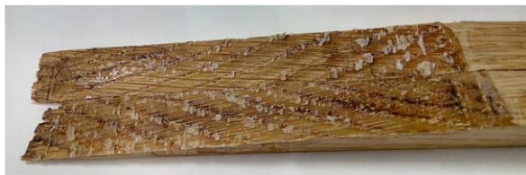
Figure 5: Localized micro wood failure mechanisms (Scekic, 2018).
