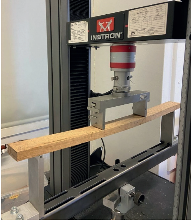
Figure 2: Four-point bending setup with s/l = 3 .
