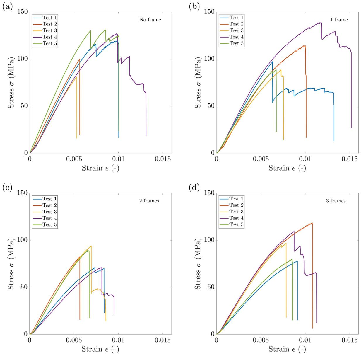
Figure 3: Stress-strain curves for the five repeats ( $n = 5$ ) of the four-point bending tests with (a) no frame ( $s_{CL} = 600$  mm), (b) 1 frame ( $s_{CL} = 300$  mm), (c) 2 frames ( $s_{CL} = 200$  mm) and (d) 3 frames ( $s_{CL} = 150$  mm).
