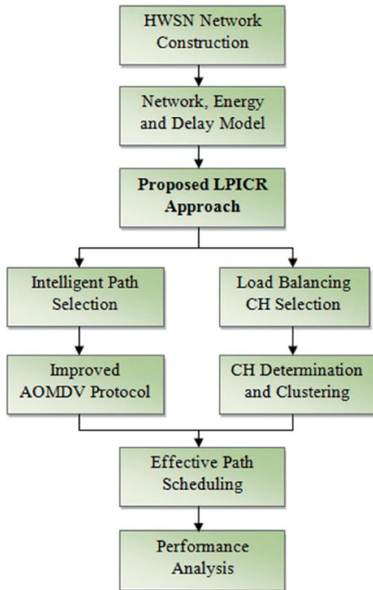
Figure 3. Work flow of proposed LPICR-HWSN
