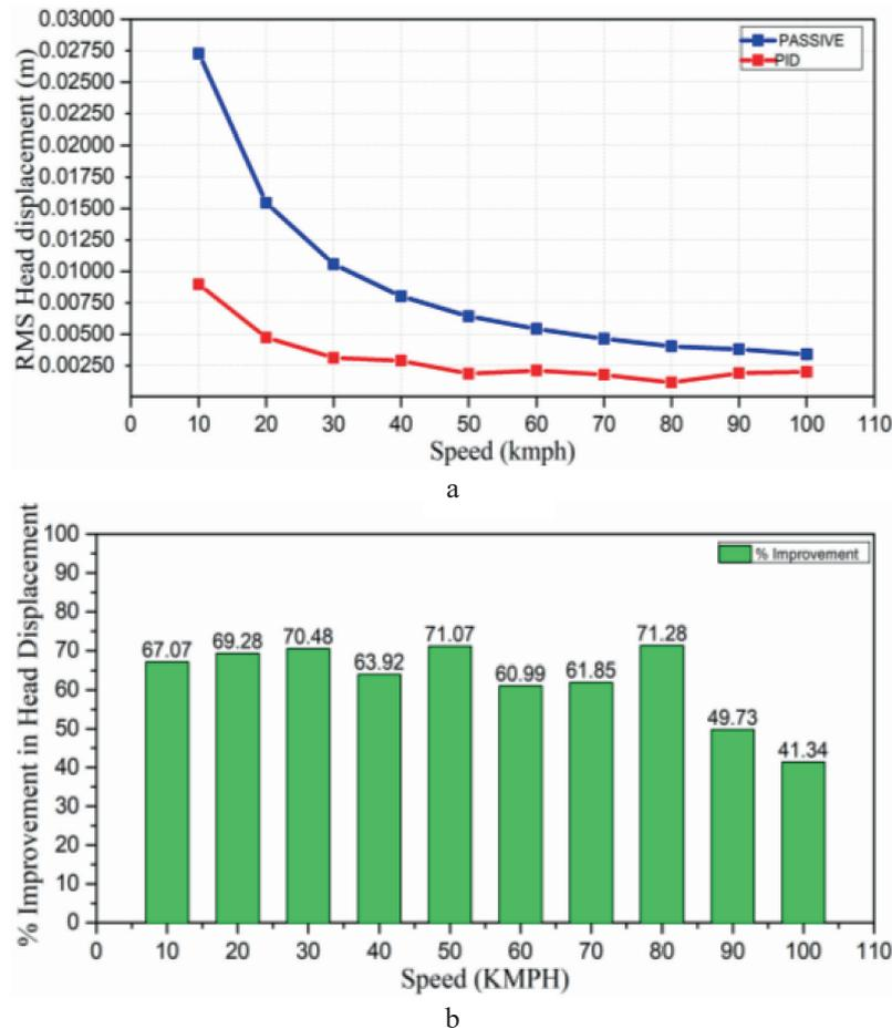
Figure 9. Head displacement improvement using PID (a) RMS (b) % improvement
