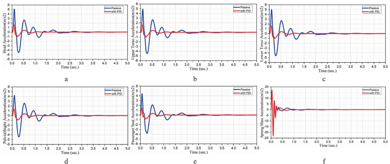
Figure 6. Acceleration response (a) Head (b) Upper Torso (c) Lower Torso (d) Pelvis (thigh) (e) Seat and (f) Sprung mass at 40 km/h
