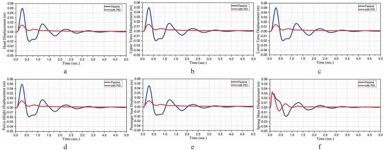
Figure 7. Displacement response (a) Head (b) Upper Torso (c) Lower Torso (d) Pelvis (thigh) (e) Seat (f) Sprung mass at 40 km/h
