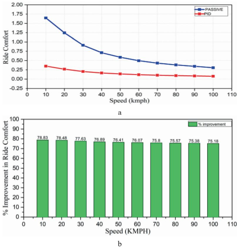
Figure 8. Ride Comfort improvement using PID (a) RMS (b) % improvement
