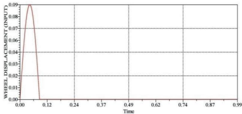
Figure 5. Sinusoidal road profile bump used for simulation
