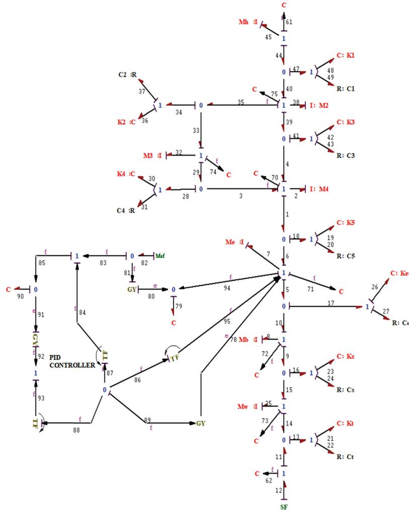
Figure 4. Integrated 7-DOF Active suspension quarter car Bond Graph model with PID controller
