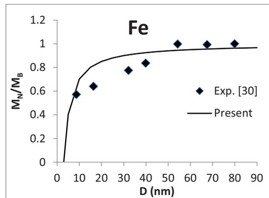
Figure 1. Relative magnetization versus diameter in Fe (Sphere) nanomaterial
