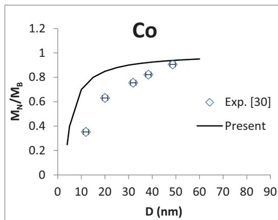
Figure 3. Relative magnetization versus diameter in Co (Sphere) nanomaterial
