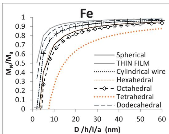
Figure 8. Relative magnetization with size for Fe nanosolid of different shapes
