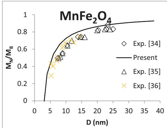
Figure 6. Relative magnetization versus diameter in  $MnFe_2O_4$  (Sphere) nanomaterial
