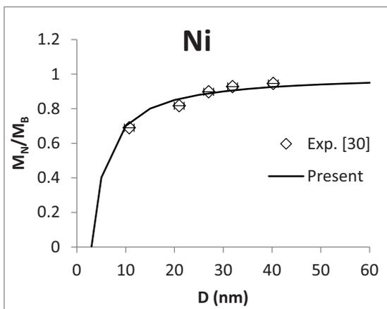
Figure 2. Relative magnetization versus diameter in Ni (Sphere) nanomaterial
