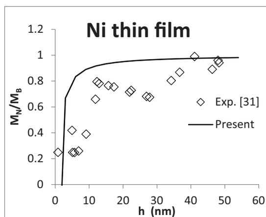
Figure 4. Relative magnetization versus size in Ni (thin film)
