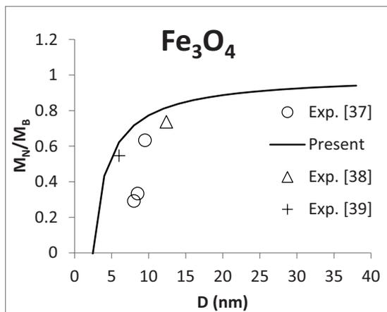
Figure 7. Relative magnetization versus diameter in  $Fe_3O_4$  (Sphere) nanomaterial
