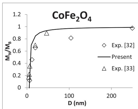
Figure 5. Relative magnetization versus diameter in  $CoFe_2O_4$  (Sphere) nanomaterial
