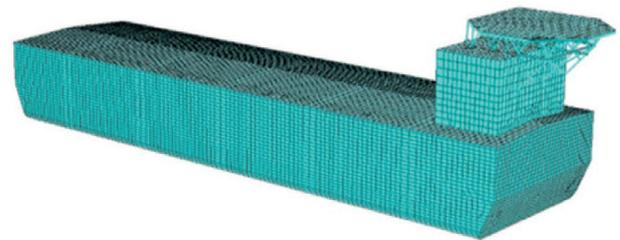
Figure 16. SE-23 FPSO model (Sample model)
