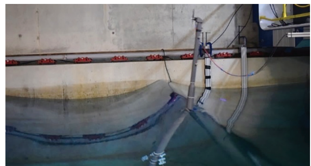
Figure 21. Effect of a rogue wave on a moored floating wind turbine model. A propeller is used to represent the wind turbine thrust.
