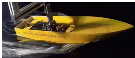
Figure 6. Wave pattern of bare hull model (exp) at F_n = 1.78
