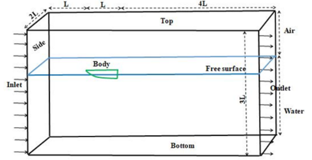
Figure 2: Schematic diagram of computational domain with boundary conditions.
