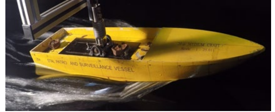
Figure 6: Wave pattern of bare hull model (exp) at F_n=1.78
