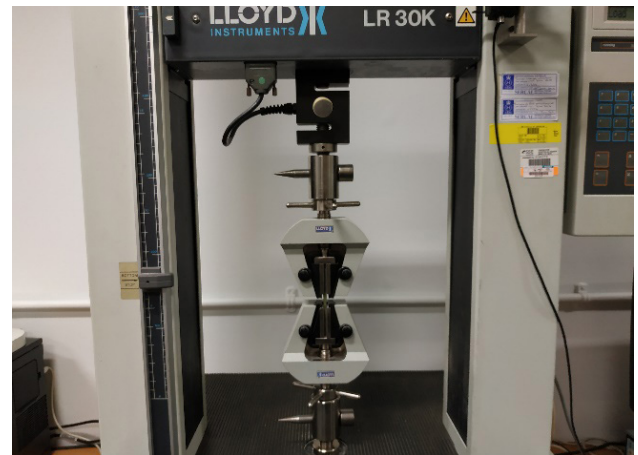
Figure 1. Experimental setup (compressive test) on a Lloyd Instruments LR30K (Wisniewski, 2019).
