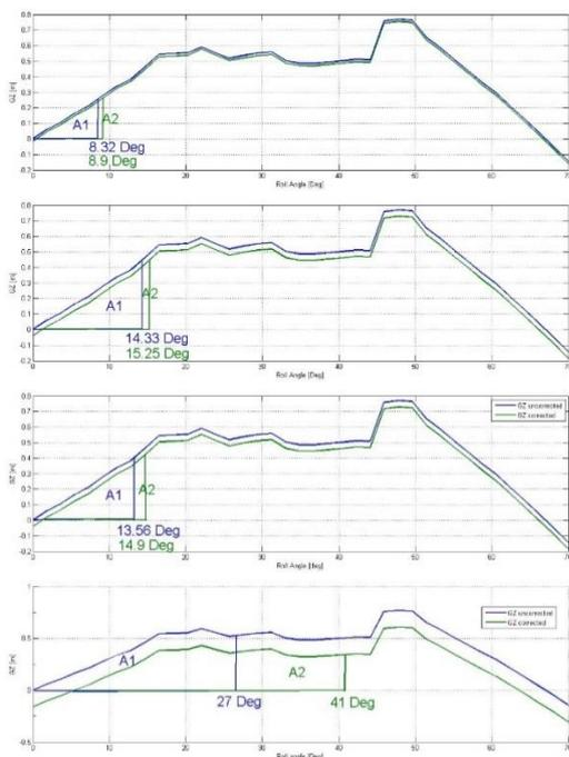
Figure 16. Correction of righting arm curve due to maximum possible impact from sloshing force in investigated flooded compartment
