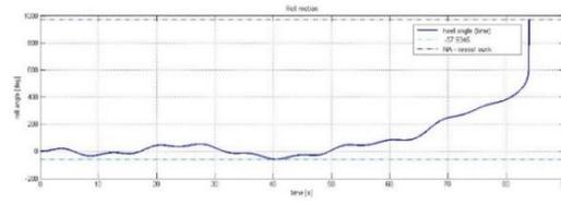
Figure 12. Hs=4m, Tn=8 sec – Roll motion (vessel capsized due to excessive heeling force)
