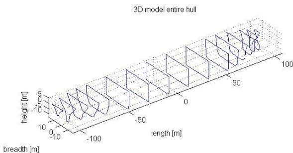
Figure 1. Isometric view of the hull of oil tanker type Szczecin II
