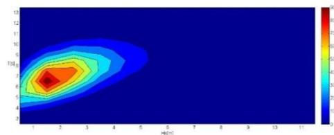
Figure 2. Frequency distribution of sea states in function of wave periods and significant wave height for worldwide trade. (Total number normalized to 1000) (Cramer, 1994)
