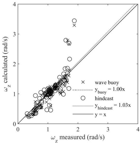
Figure 2: Comparison of stress zero-crossing frequencies calculated with wave buoy and hindcast data against zero-crossing frequencies derived from strain gauge measurements.
