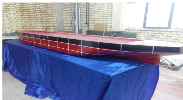
Figure 2. Painted and scaled model of the SALINA
