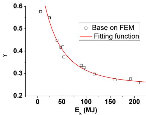
Figure. 9 Kinetic energy reduction factor by fitting power function
