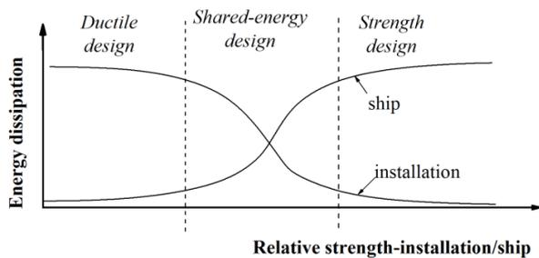
Figure. 3 Design principles base on relative strength
