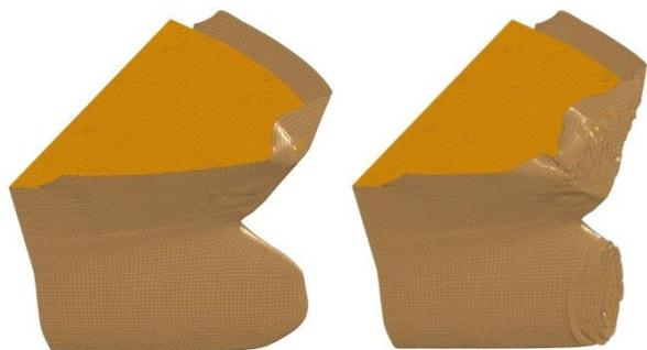
(a) Crush of the upper deck (b) Crush of the upper deck and bulb bow
