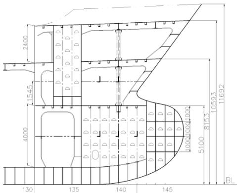
Figure. 1 Section of the ship bow
