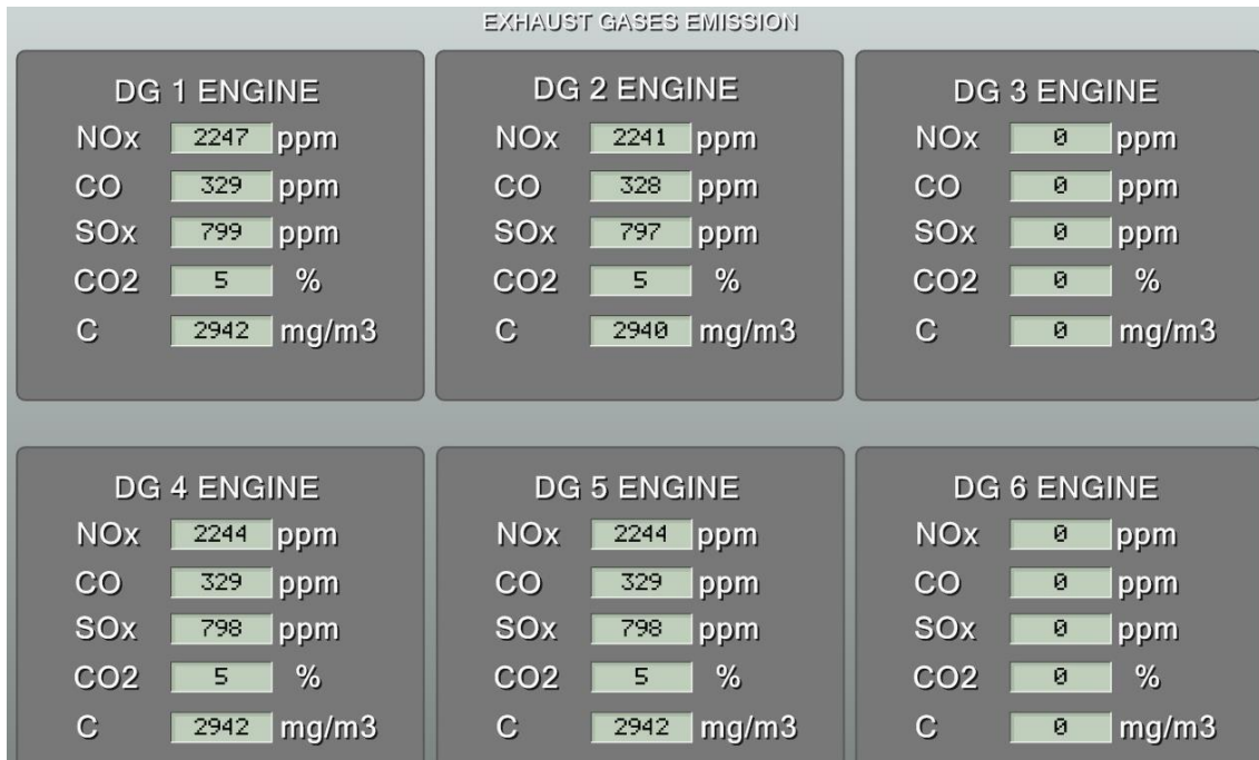
Figure.4b. Four-generator emissions quantity
