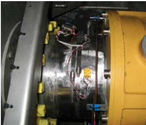
Figure 2: SKM shaft power instrumentation on Hull 064 112m wave-piercing catamaran (Gillespie, 2007).
