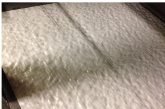
Figure 7: Scaled replica of “orange-peel” pattern from freshly cleaned and painted Dharma Kencana IX ship hull inside a wind tunnel
