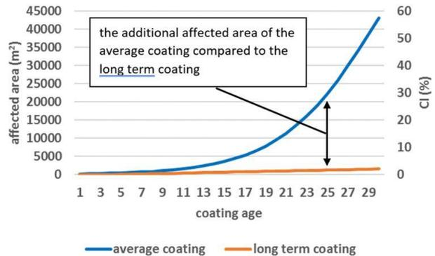
Figure 4: Regression curves of the average coating degradation versus the long term coating degradation expressed in affected area (considering 90,000m ballast tank area) and expressed in CI.
