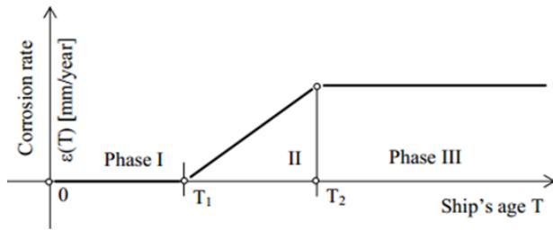
Figure 2: Corrosion rate versus ship's age, 3 distinctive phases. Phase I: no corrosion wastage, phase 2: gradual acceleration of corrosion, phase III constant corrosion rate (Lyuben et al., 2003)
