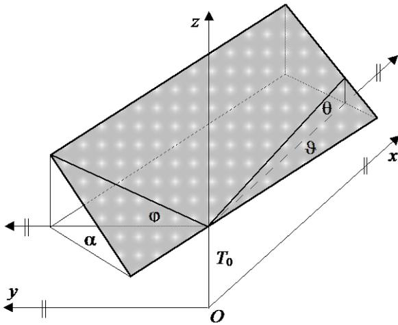
Figure 5. Analytical angles of inclined waterplane
