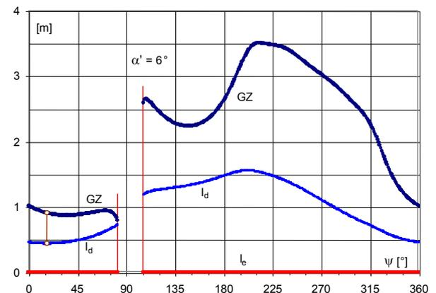
Figure 27. Run of righting arm  $GZ$  and dynamic arm  $l_d$  for rig versus twist  $\Psi$  for heel angle less than critical
