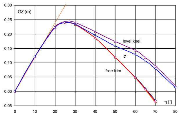
Figure 17.  $GZ$ -curves of the fishing boat
