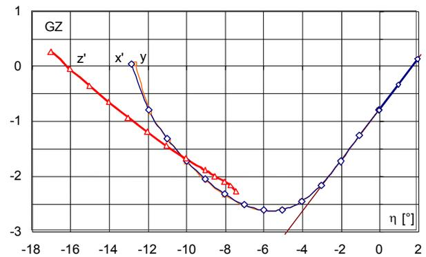
Figure 25.  $GZ$ -curves of rig for inclinations to portside
