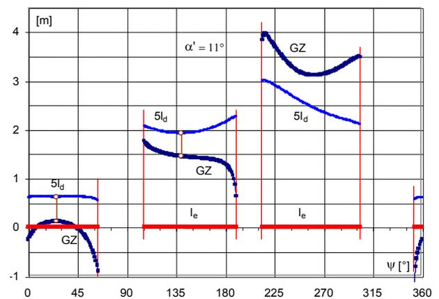
Figure 23. Run of the righting arm  $l$  and dynamic arm  $l_d$  for rig versus azimuth  $\Psi$  for  $\alpha' = 11^\circ$  for reference axis  $Oy'$
