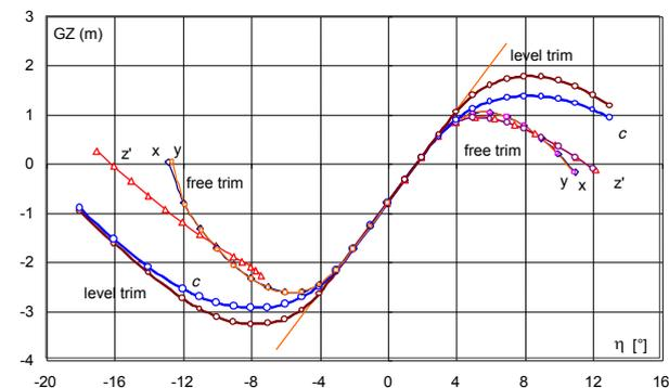
Figure 26.  $GZ$ -curves of rig for inclinations to both sides
