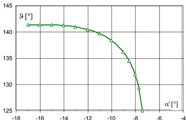
Figure 21. Run of twist around axis  $Oz'$  during heeling rig to portside
