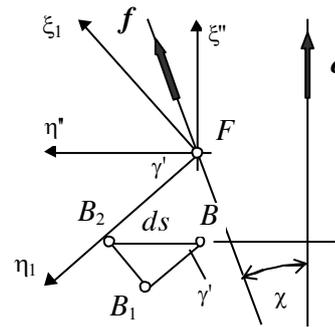
Figure 13. Components of shift of centre of buoyancy in the principal co-ordinate system  $\xi_1\eta_1$
