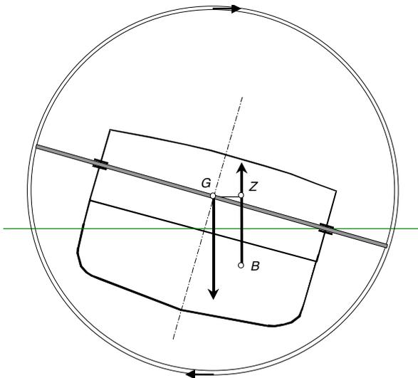
Figure 3. Oblique trimming around the y-axis
