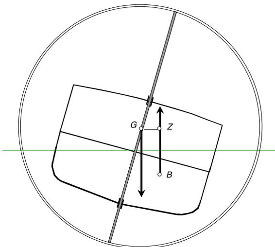
Figure 4. Oblique trimming around the z'-axis
