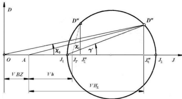
Figure 12. Mohr's circle and stability characteristics
