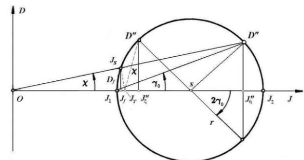
Figure 11. Principal direction and transverse moment of waterplane inertia  $J_T$
