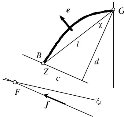
Figure 15. Projection of curve of centres of buoyancy on the waterplane
