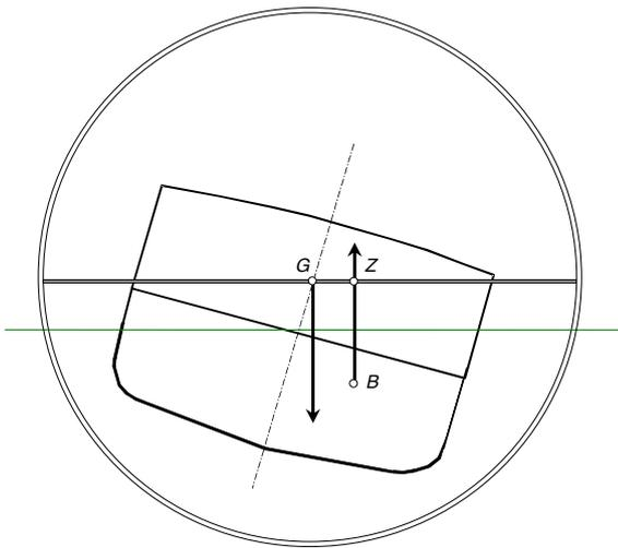
Figure 2. Vertical trimming of the ship
