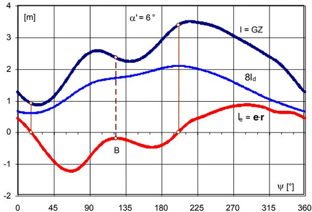
Figure 24. Run of stability characteristics  $l$ ,  $l_e$  and  $l_d$  for rig versus azimuth  $\Psi$  for  $\alpha' = 6^\circ$
