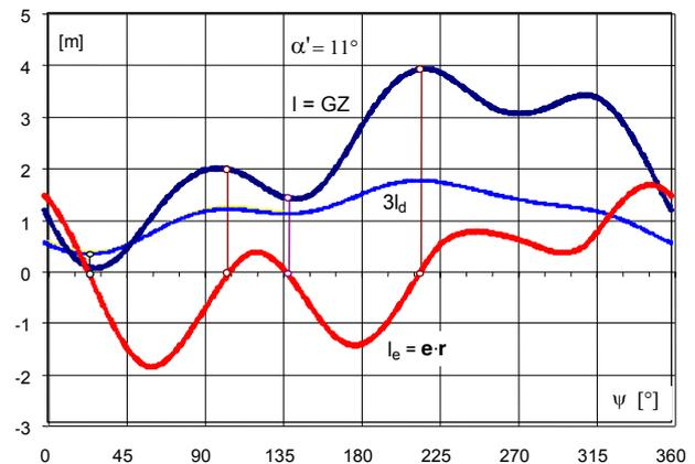
Figure 22. Run of stability characteristics  $l$ ,  $l_e$  and  $l_d$  for rig versus azimuth  $\Psi$  for  $\alpha' = 11^\circ$  for reference axis  $Oz'$
