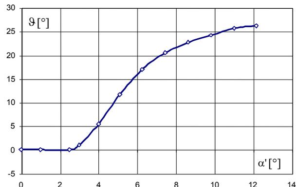
Figure 20. Run of twist around axis  $Oz'$  during heeling rig to starboard
