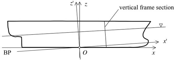
Figure 6. Co-ordinate system for a trimmed vessel
